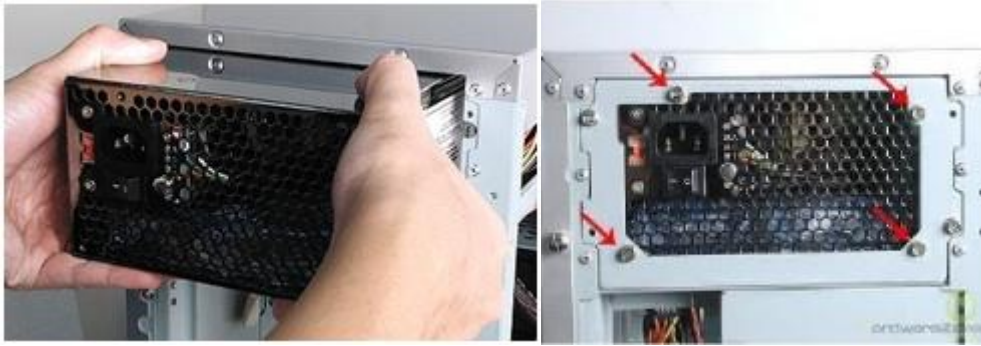
(Gambar 1.5) Cara memasang power supply
