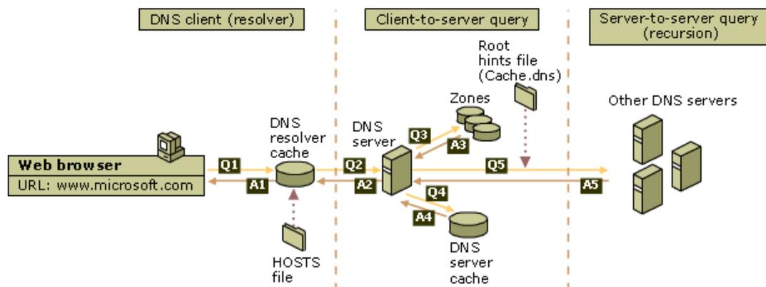
13.2. Gambar 2. Cara kerja DNS Resolver
