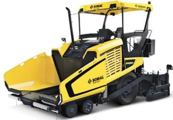
Gambar 1.16 *Asphalt finisher*
